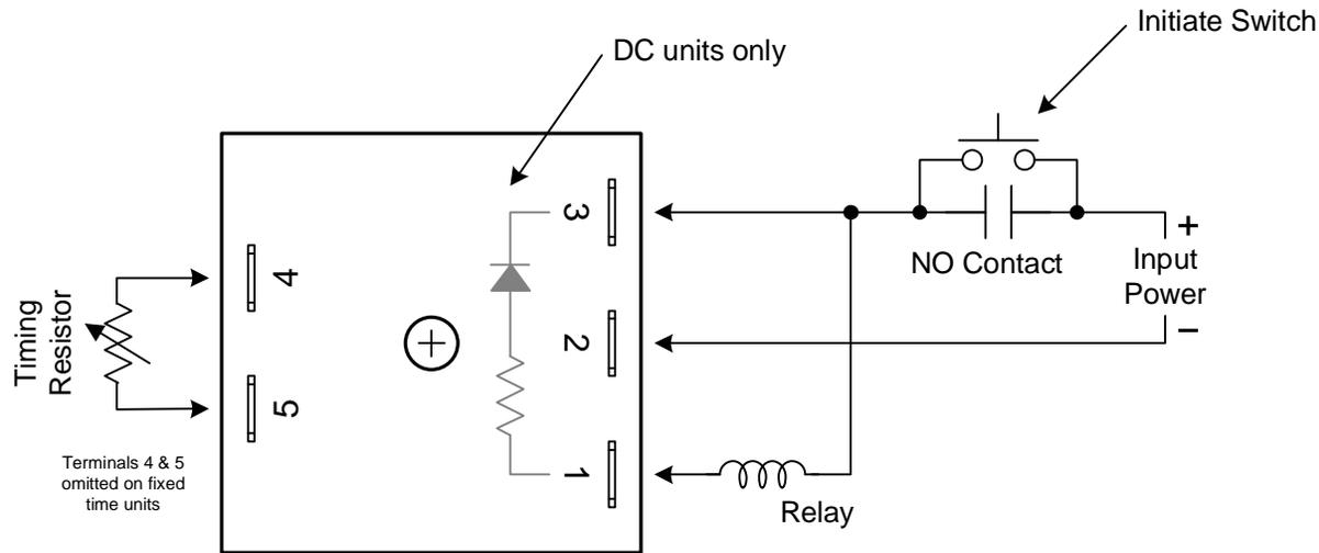
Requires momentary switch to initiate time delay and one normally open contact set on load relay.
